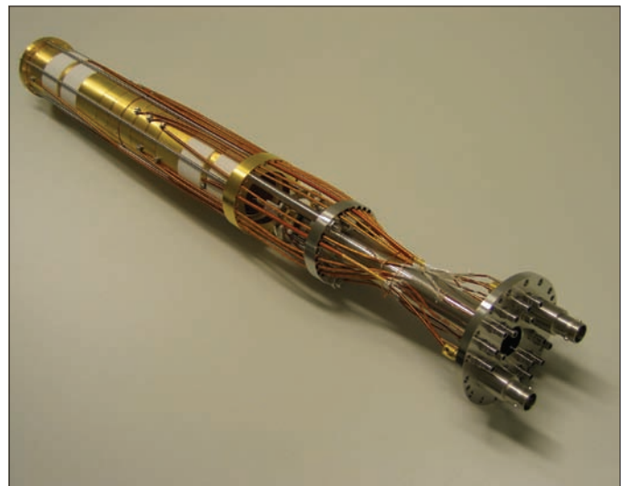
Fig. 1. ALPHA's Penning trap for catching antiprotons from CERN's AD. The stack of gold-plated electrodes is placed in a cryostat inside a superconducting solenoid magnet generating a field of up to 3 T. (Courtesy N Madsen/Swansea.)
