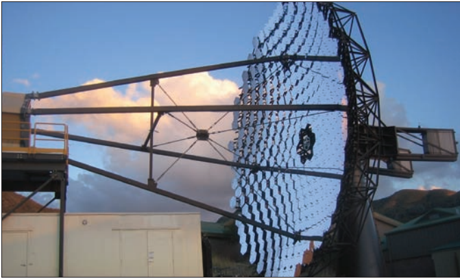
One of the four VERITAS 12m telescopes near Mount Hopkins in Arizona, showing the camera box, tessellated mirror and counterweights. (Courtesy David Hanna, McGill University.)
